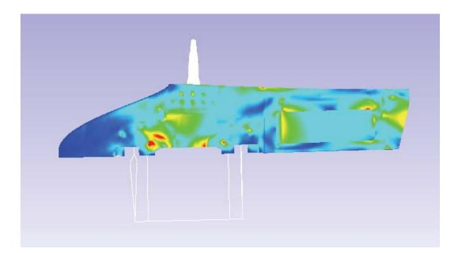
Critical element location within the most "heavy" load condition
