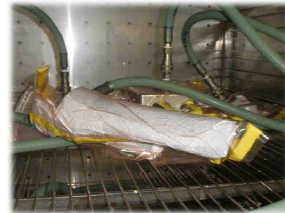
Thermal cure of vacuum-bagged composite part.
