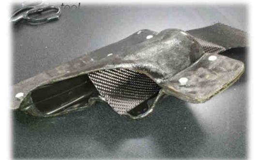
Pull composite strips through tool and press against walls.
