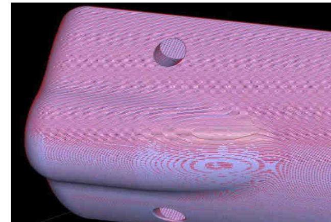
Consider small slice heights for fine features.
