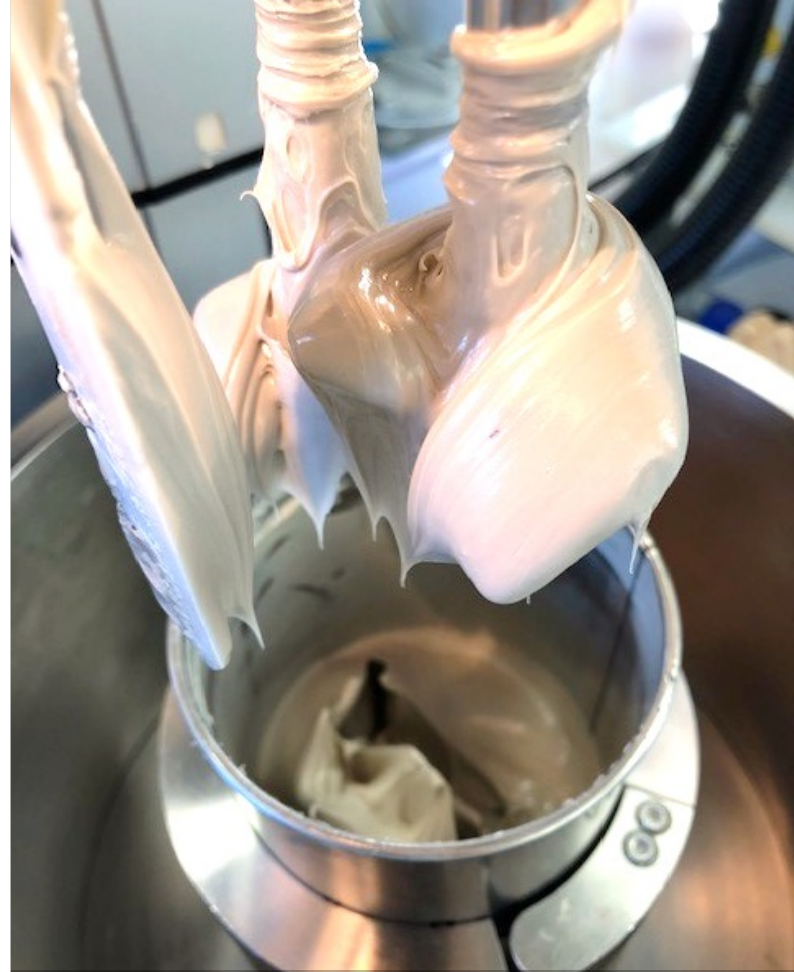
Picture of generic formulation. Thioplast™ EPS35 starting formulation visco.: 14-18 Pas.
